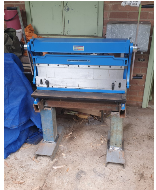
Above: The stand made by Ken Baker to mount the new rollers.
