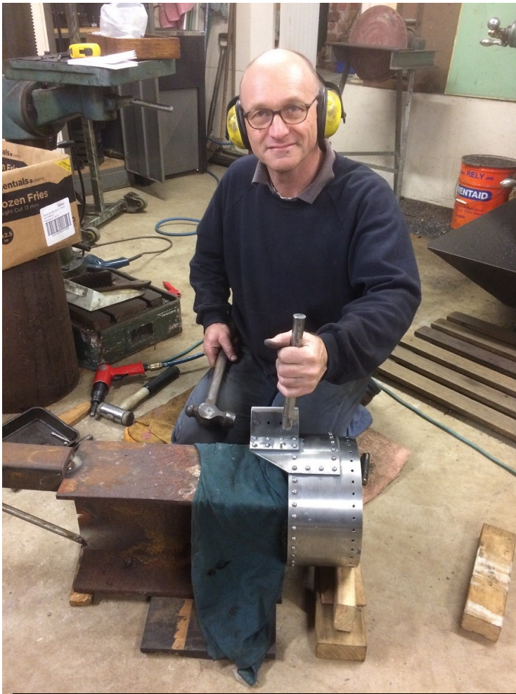
Pounding 3/16" steel rivets into the smokebox.
